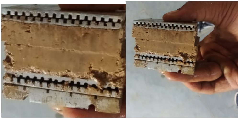
Figure 18 : Shows Direact Shearing of the Soil Sample (samples from the Dump)
