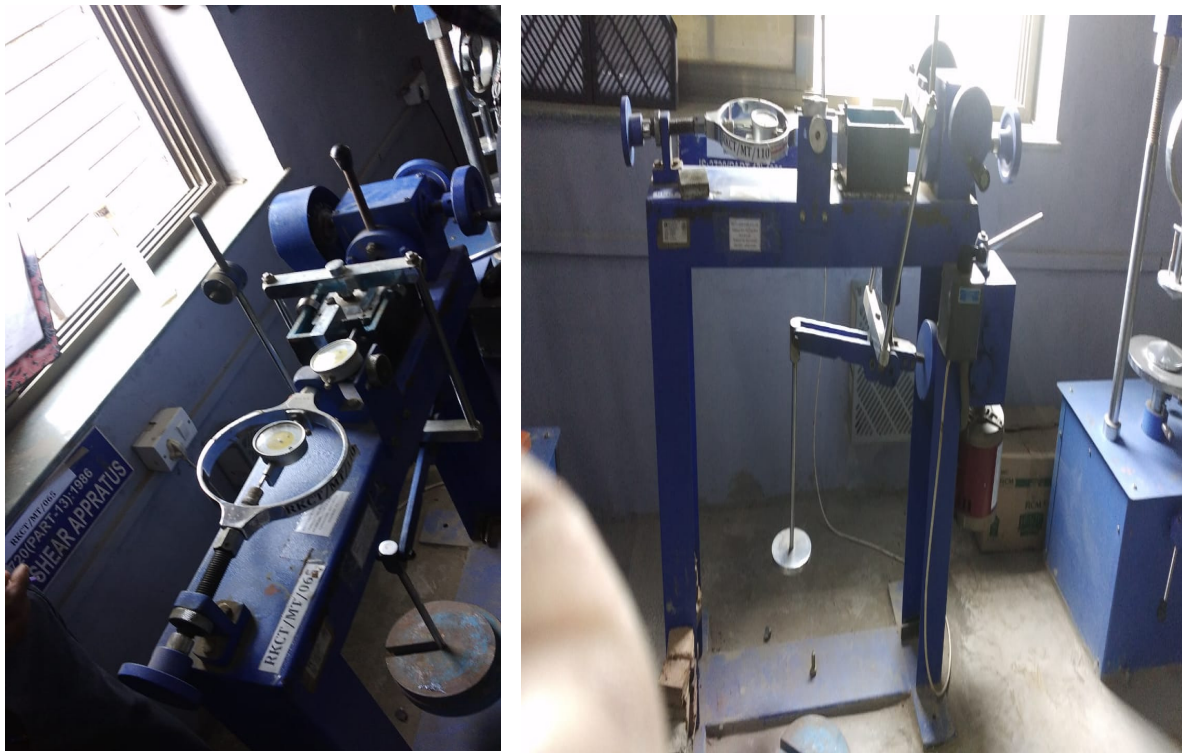
Figure 17 : Shows Direct Shear Strength Testing Unit
